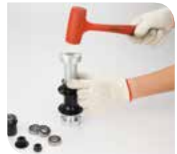
15 Install the bearing with rubber hammer
