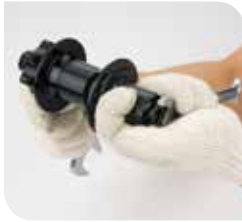
1 Un-tighten the lock-nut by wrench
