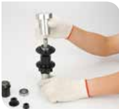
18 Take the holding tool (B) onto the bearing (drive side)
