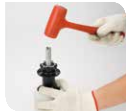
10 Push the other bearing out by rubber hammer
