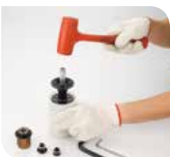
7 Push out the bearing out of the freehub by rubber hammer
