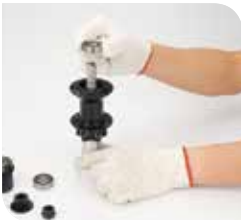
17 Take one bearing on the axle (drive side)
