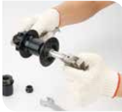
3 Un-tighten the lock-nut by disassembly tool with wrench
