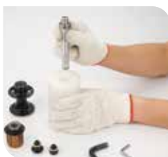
9 Put the axle down to the holding tool (A)
