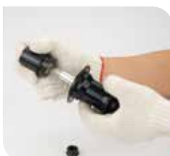
23 Slide the new Freehub Body inside the axle
