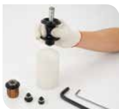
6 Put down the hub on holding tool (A)
