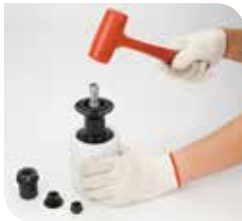
6 Push out the bearing by rubber hammer
