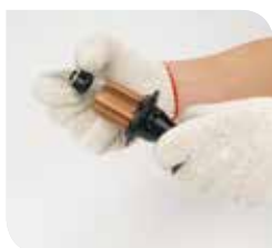
26 Threaded the alloy end cap in drive side
