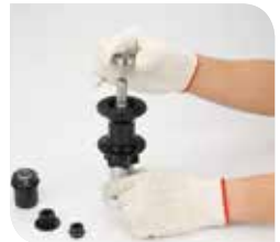
20 Take the other bearing for drive side
