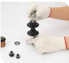
13 Put the bearing on non-drive side
