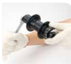
24 Threaded the lock-nut (drive side)
