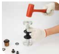
15 Install the bearing with rubber hammer
