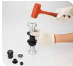
19 Install the bearing with rubber hammer
