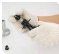
24 Threaded the end nut from non-drive side
