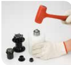
8 Push out the bearing by rubber hammer
