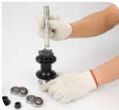
12 Put the axle inside the hub shell
