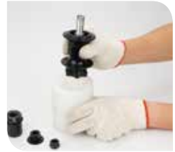
5 Put down the hub (disc side) on holding tool (A)
