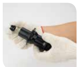
25 Tighten the lock-nut (drive side) with wrench
