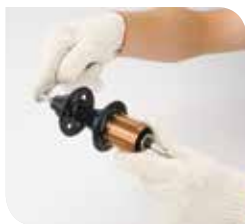
1 Un-tighten lock-nut from non-drive side
