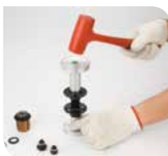
19 Install the bearing with rubber hammer
