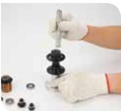
12 Put the axle inside the hub shell
