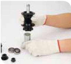
16 Put down the hub on holding tool (C)
