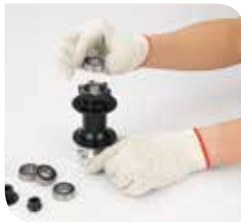
13 Take on bearing onto hub shell (disc side)
